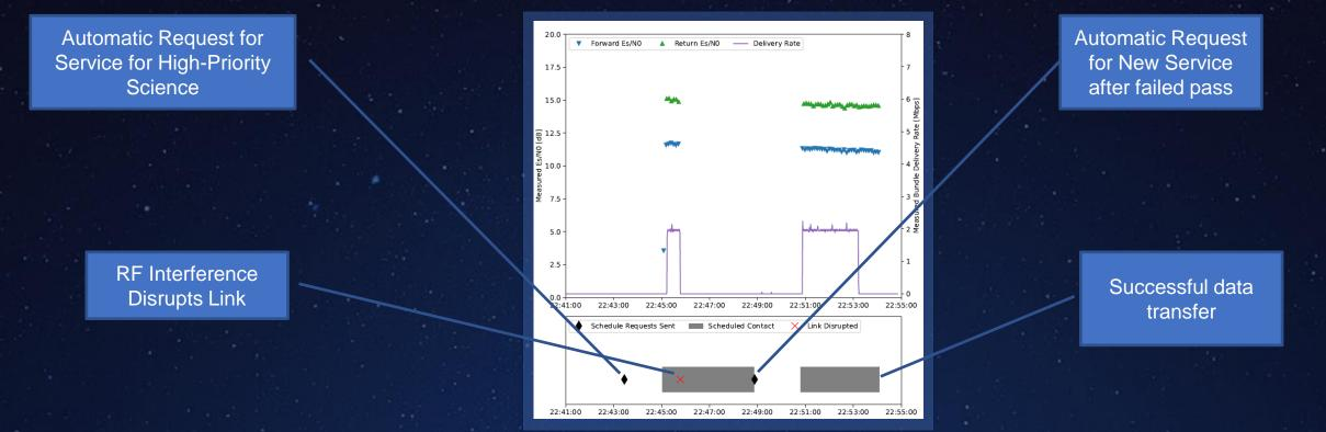
Initial demonstration demonstrates core functionality of the testbed, including end-toend DTN data flow, automated operations of the testbed, and supporting testing of autonomous/cognitive communications systems, without human interaction.
