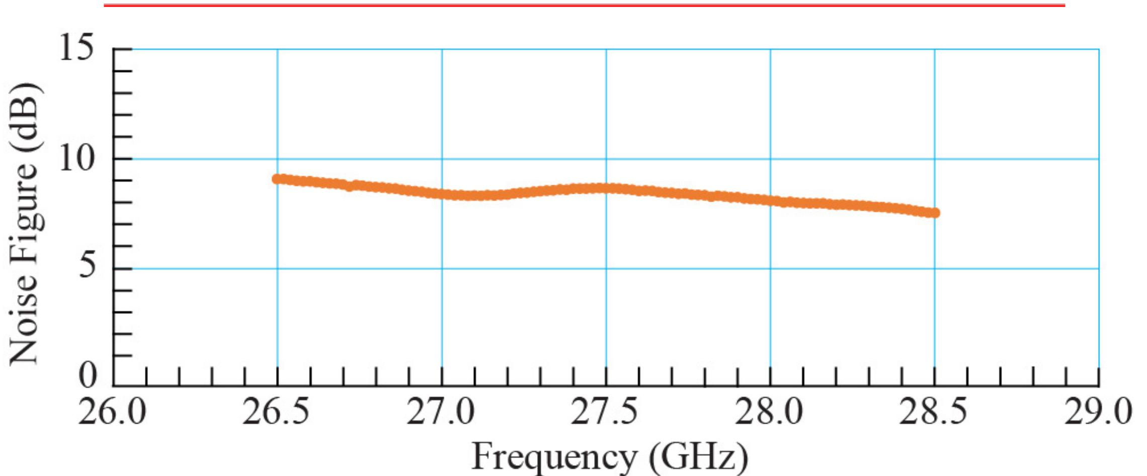
✓ In a cognitive radio while transmitting a HPA with low noise figure ( $\leq 9.0$  dB) implies less S/N ratio degradation of the adjacent channels and while receiving less deviation of the constellation points from their desired locations
