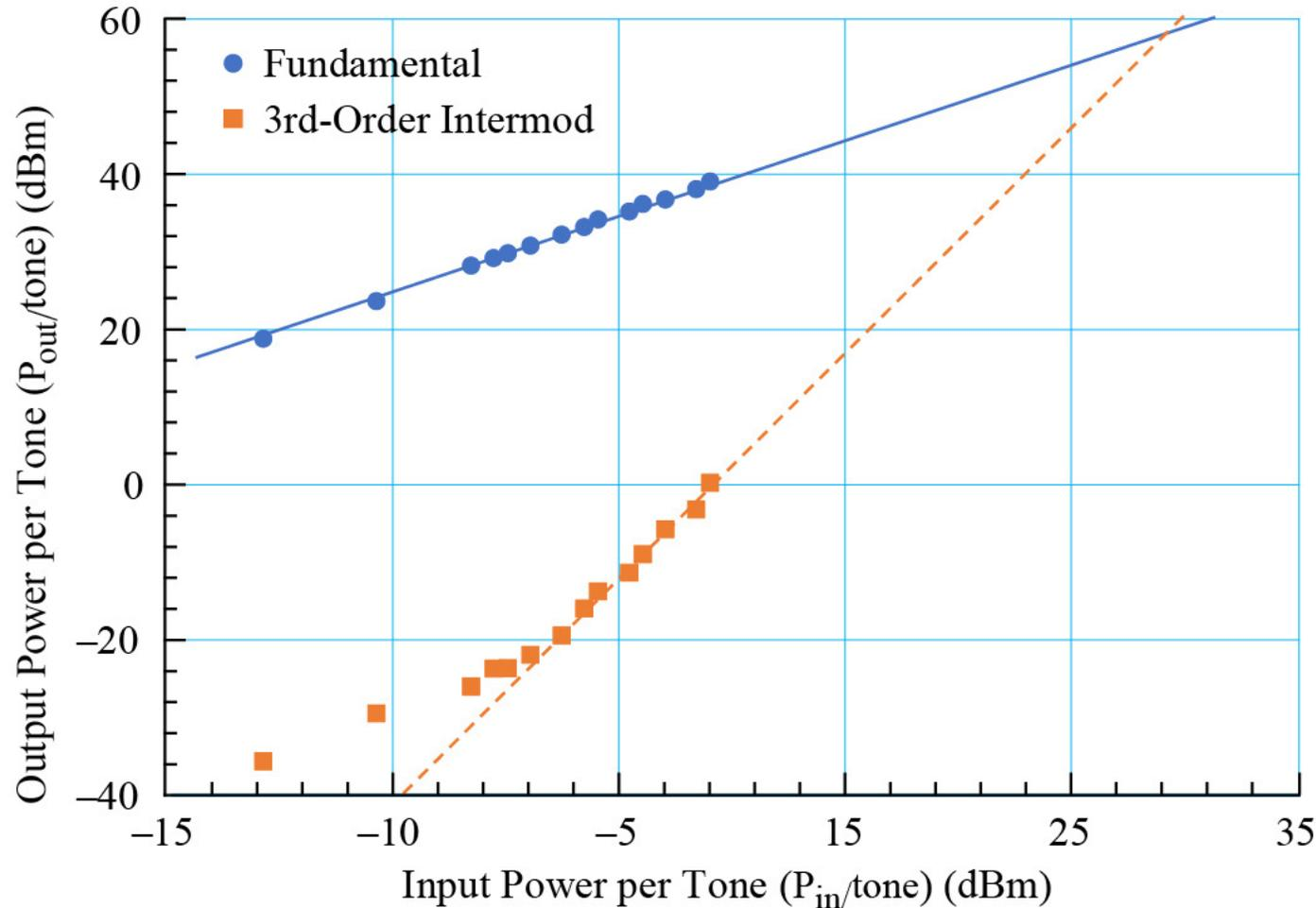
✓ The high OIP3 on the order of 56 dBm demonstrated that the 3rd-order IMD products generated by the HPA is small. Therefore, the interference signals generated within the cognitive radio channel bandwidth due to HPA nonlinearity is also small
