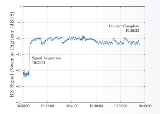
Relative power of ADC samples shows averaging effect of receiver automatic gain control.
