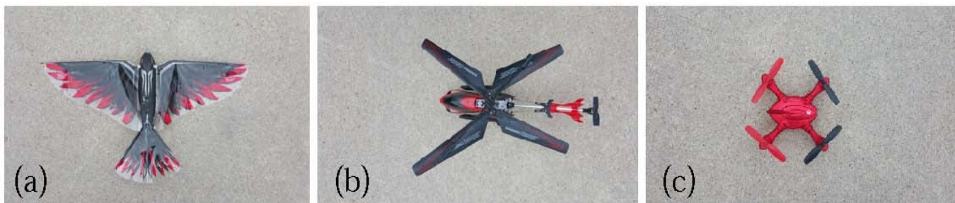
Figure: Images of the drone objects used for the experiment: a) Air Hog Firewing (UAS1); b) Sky Rover Cop (UAS2); c) Radioshack Surveyor (UAS3).
