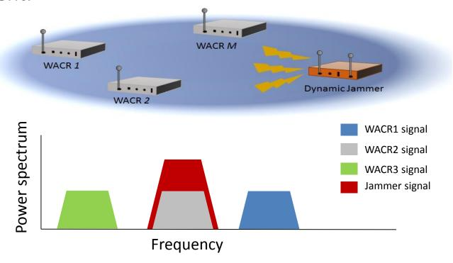
• Goal: find optimal anti-jamming and interference avoidance policies for the WACRs that switches transmission before getting jammed.
