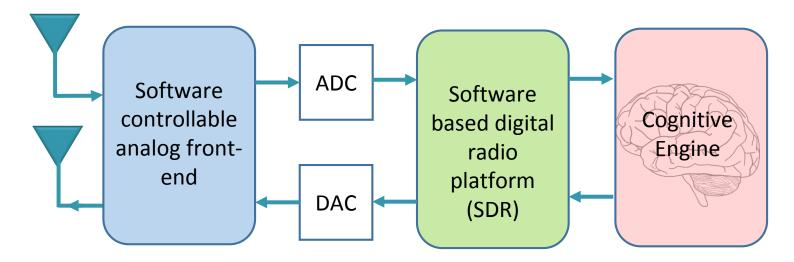
A cognitive radio is a multiband, multimode, wideband software-defined radio (SDR) with autonomous decision-making and learning abilities that can optimally reconfigure its operation mode in response to its surrounding RF environment and user needs.
