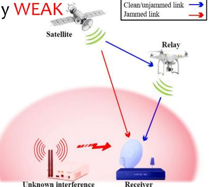
Solution: new entities, e.g., unmanned aerial vehicles (UAVs, or drones) can be used to assist such corrupted links (No modification or reconfiguration to the ground or satellite) University of South Carolina
