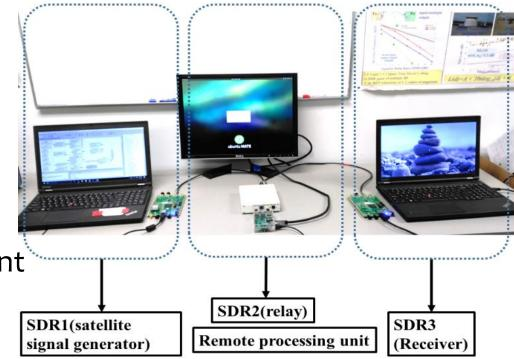
Contains three SDRs, working as transmitter, relay, & receiver
