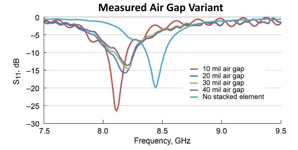
\*The main takeaway from this experiment is that the central frequency in a stacked square patch can be reconfigured by as much as 100MHz (Shifted from 8.1017 to 8.2017 GHz).
